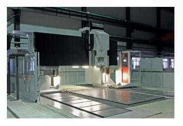
MATEC 30PB | 40PB | 50P Machine table/clamping surface on hall floor level | Fully accessible | Profitable for high and heavy workpieces
