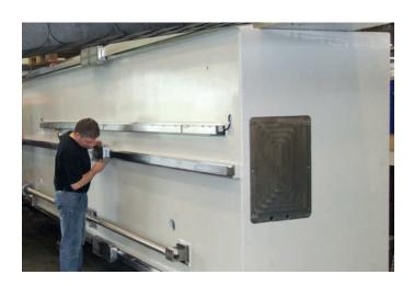
The gantry cross-section is significantly larger in the diagonal than the travel of the Z-axis. Thereby deformations due to bending and torsion are reduced to barely measurable values.
