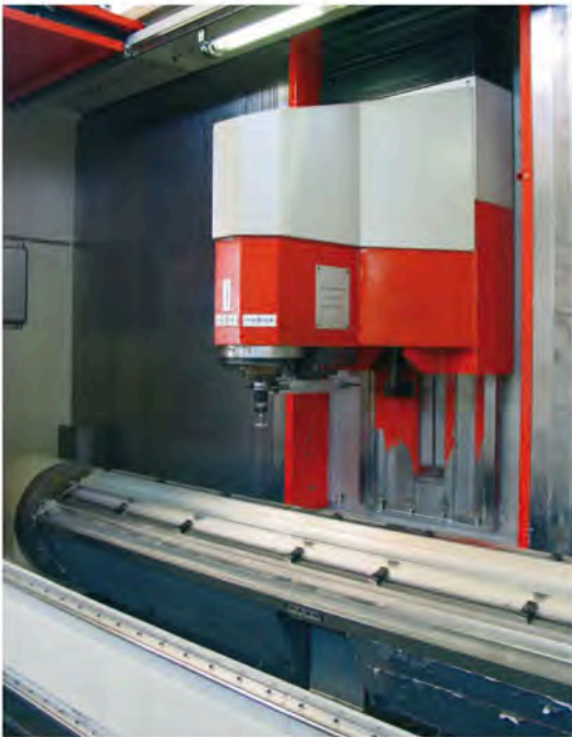
Left: matec-30 L, working area with mounted rotary table. Machining of aluminium profiles.
