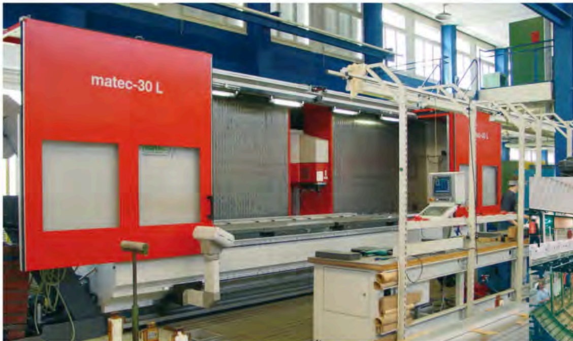
CNC traveling column machining center matec-30 L with traverse paths of X = 6.000 mm, Y = 800 mm and Z = 800 mm for the flexible complete machining of parts of all sizes
