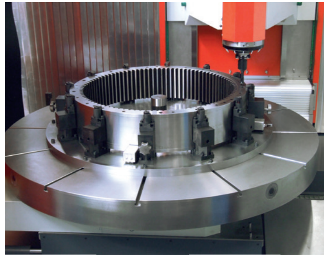
Balancing of workpieces on the mill turn centre For balancing rotationally symmetrical workpieces. The position and size of the unbalance are determined automatically.
