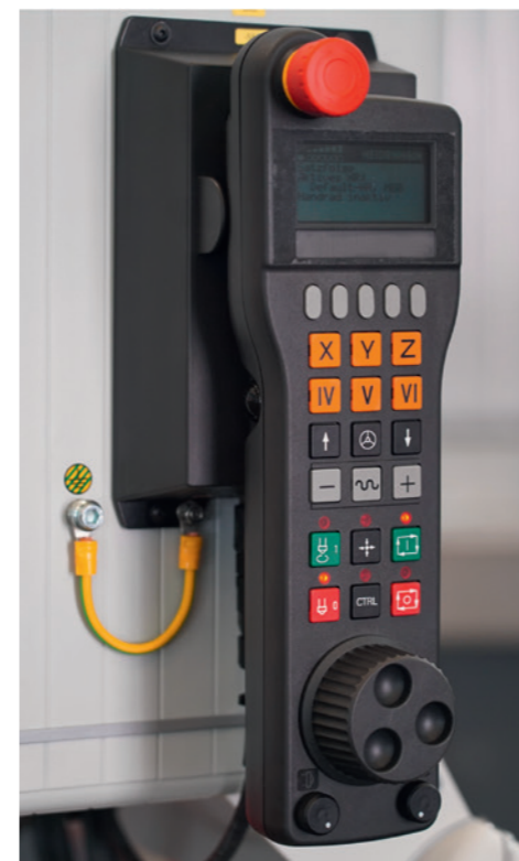
Handwheel for manual operation of machine tools. Version with cable or via radio.
