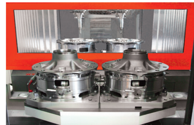
Work area 1: Loading station. Hydraulically operated double clamping device for automation.
