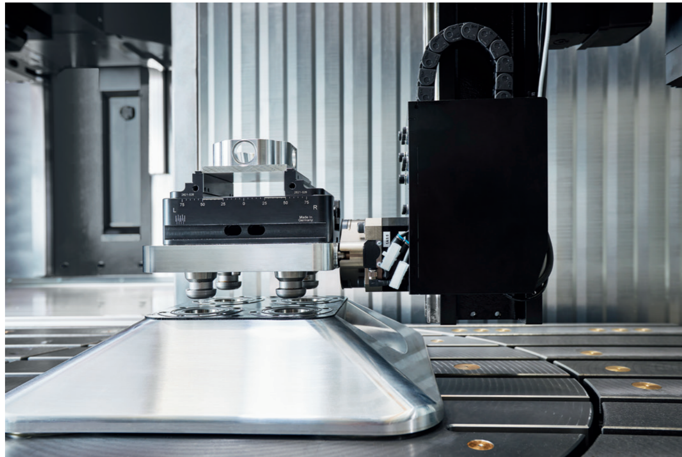
Basic fixture for automation on the rotary table. Workpiece pallet clamping via zero-point clamping system. Pallet sizes ranging from 150 x 150 mm to 800 x 800 mm.
