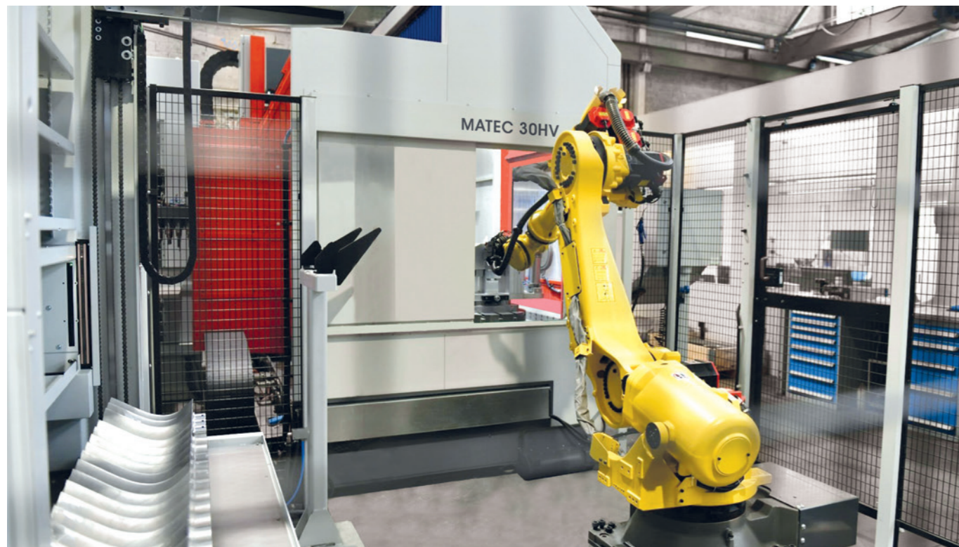
5-axis series production of turbine blades.
