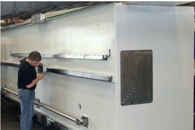
**The gantry cross-section** is significantly larger in the diagonal than the travel of the Z-axis. Thereby deformations due to bending and torsion are reduced to barely measurable values.
